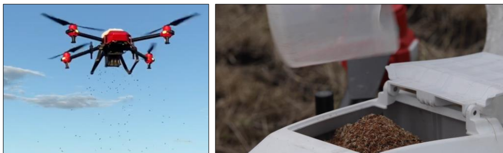
Figures 20-21 – Drone seeding, and seed spreader being filled (Source: XAG Australia 2020).
